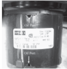
Figure 22. Oil ports on a circulation fan
