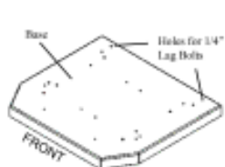
Figure 16A BayWin Anchor Holes
